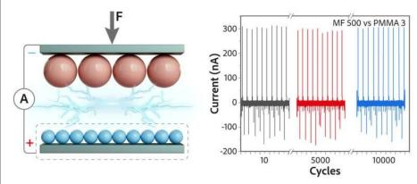
Schematic representation of the working of triboelectric nanogenerator surfaces. Credit: Ignaas Jimidar
