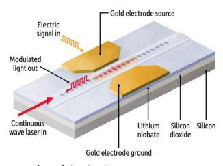
A schematic drawing shows an electro-optical modulator developed in the lab of Qiang Lin, professor of electrical and computer engineering. The smallest such component yet developed, it takes advantage of lithium niobate, a "workhorse" material used by researchers to create advanced photonics integrated circuits. (University of Rochester illustration / Michael Osadciw)
