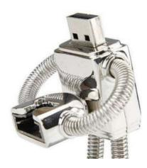
There is a limit to the number of times a flash drive's transistors can be switched from one electrical state to another; eventually, it will become impossible to write data to an exhausted transistor. In one hands-on test, this limit was found to be over 90 million write operations! Interestingly, the data already on the tested flash drive could still be read even when writing new data to it was no longer possible. Data was not lost.
