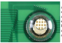
Researchers at the University of Illinois and Northwestern University have developed a camera with a layout similar in size and shape to the human eye. The eye camera is based on "single-crystalline silicon detectors and electronics, configured in a stretchable, interconnected mesh," according to the University of Illinois.
